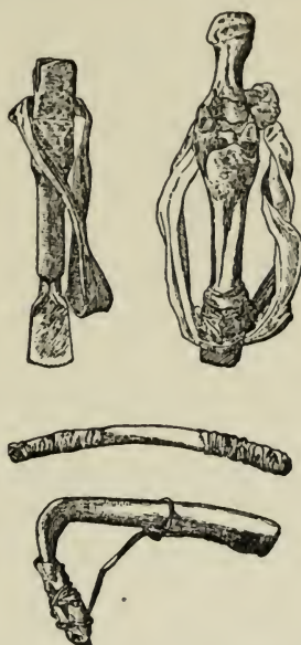
FIG. 19. CROW TANNER'S TOOL-KIT: CHISELS FOR FLESHING; BEAMING TOOL; ADZE-SHAPED SCRAPER (after Lowie)
